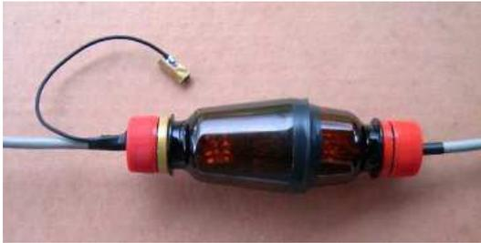
**Fig.6** Final assembly. The bottles are fixed with adhesive tape. The ground lead is short.
